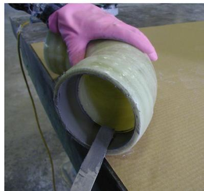
Conical surfaces may only be emerized manually. Careful use of grinding machines is permitted, but only if the pipes are installed on rollers and able to rotate.
