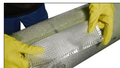
The first layer is woven roving
